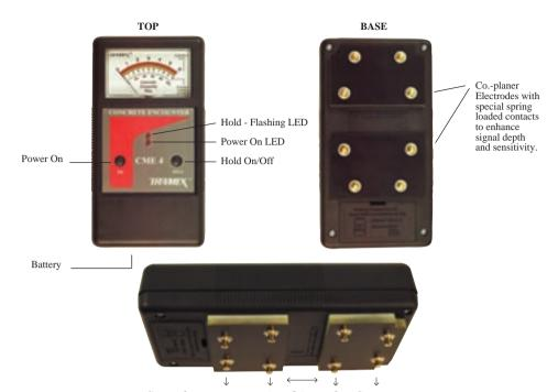
$Signals \ are \ transmitted \ into \ the \ Concrete$
